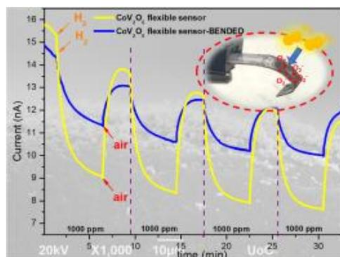
Figure 1: Gas sensing performance of flexible  $\text{CoV}_2\text{O}_6$  bended sensor towards hydrogen, operating at room temperature
