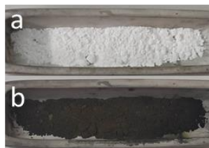
Figure 1: (a) White and (b) Black titania formed by ammonolysis
