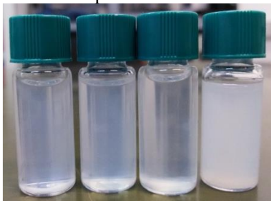
Figure 1: g-C 3 N 4 dispersions in Acetone, Acetic Acid, Butanol, Ethylene Glycol.
