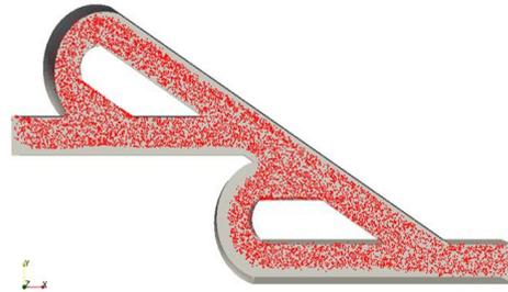
Fig. 2: Distribution of nanoparticles ( $D = 13.5 \text{ nm}$ ) into micromixer for rate equal to 1000 particles/s under  $V_p/V_c = 20$
