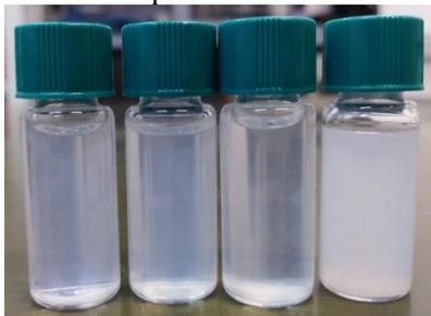
Figure 1: g-C<sub>3</sub>N<sub>4</sub> dispersions in Acetone, Acetic Acid, Butanol, Ethylene Glycol.
