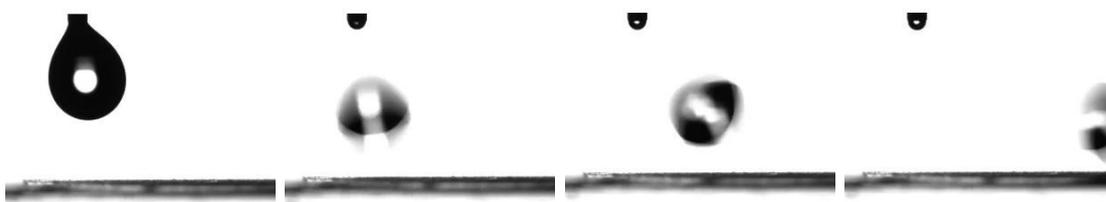
Figure 1: Water - repellent behavior of nanostructured coating deposited on LDPE substrate.
